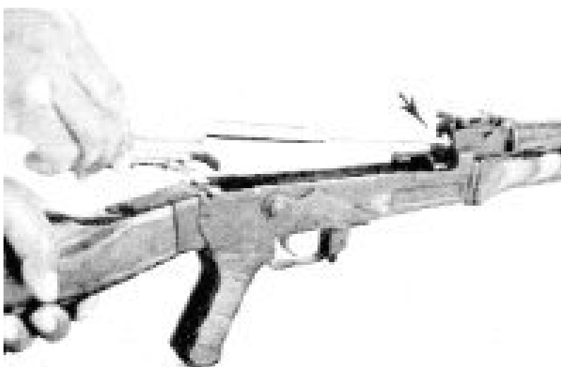
FIGURE 40. REPLACING BOLT CARRIER
